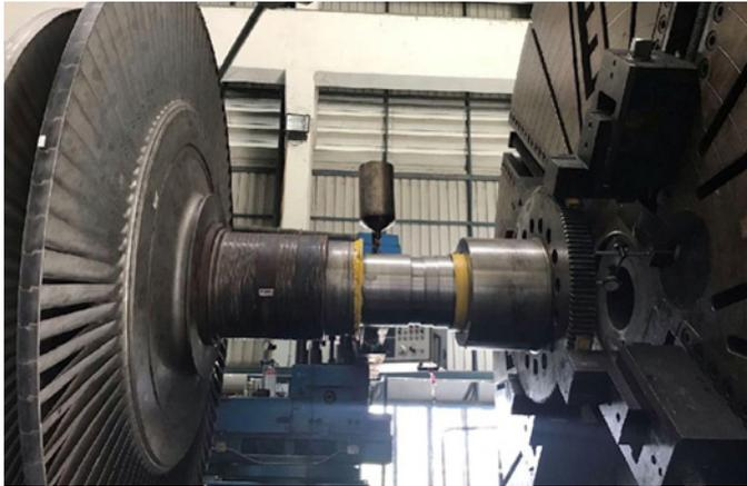
Fig. 3 • The turbine shaft mechanically prepared for welding.
