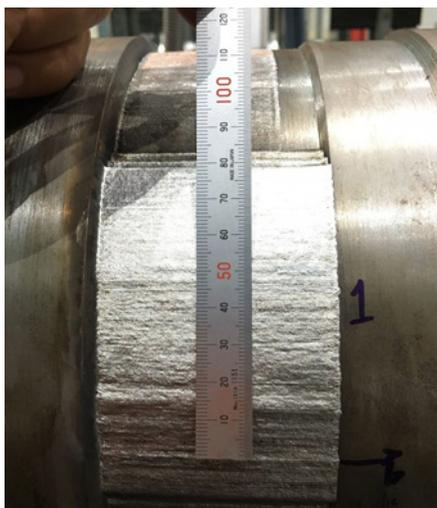
Fig. 6 • Layer structure of the pulsed laser beam repair welding.
