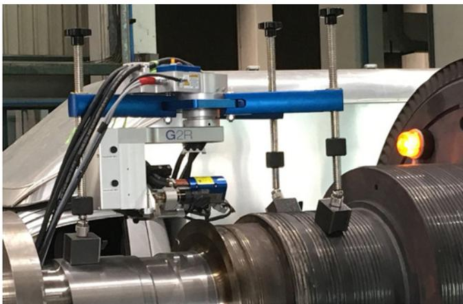
Fig. 4 • The measuring device installed before and during welding for stress testing of the turbine shaft.
