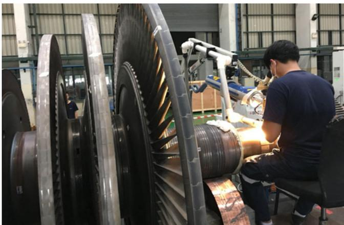
Fig. 5 • On-site welding on the turbine rotor.
